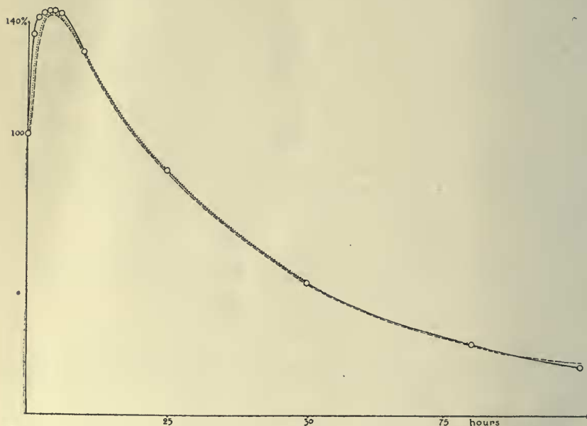
FIG. 3. Curve of electrical resistance of Laminaria in 65 NaCl + 35 CaCl 2 (————), the trial curve (-----) calculated from the velocity constants K_1 = .000481 and K_2 = .00859 , and the theoretical curve (.....) calculated from the velocity constants K_1 = .000482 and K_2 = .00859 .
